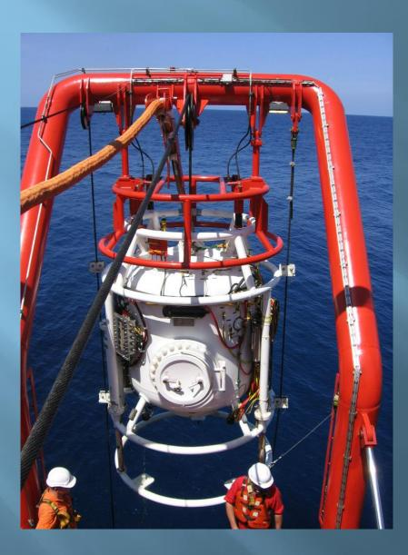
The Bell is about to be put in the water, the stand off frame ( clump weight ) has been lowered, the bell outer door is dogged and the locking hooks will be disengaged prior to lowering the bell. Looking inside a chamber you see the sound powered phone, BIBS, heater, internal depth gauge, scrubbers etc
