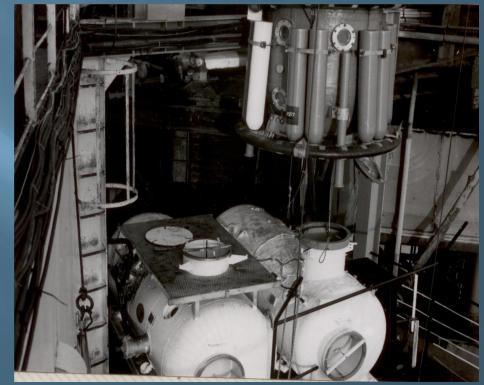
A modern modular system, note the curser, bull bars, plenty of onboard gas in case of emergency.
