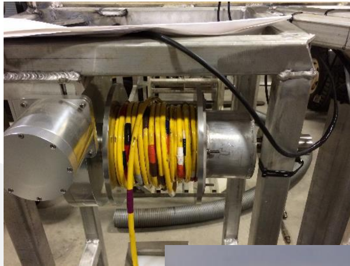
Sidescan towfish holder and winch
