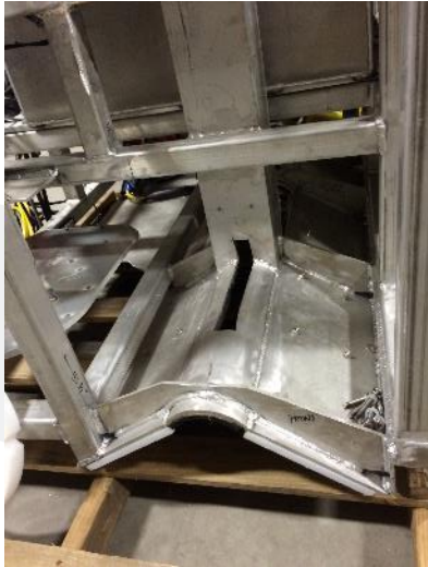
Sidescan towfish holder and winch
