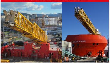
Shell Qatar operates a heave compensated Offshore Access System (OAS) onboard of one of the vessels to serve platforms in the Red Sea. The heave compensated system which maintains the end of the walkway at a constant height is automatically enabled into approach mode when the walkaway is slewed outboard from its cadle.
