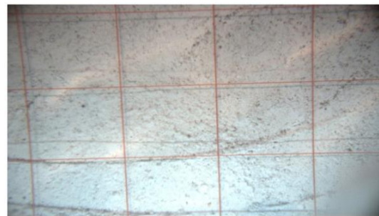
A checked frame photographed underwater with the AUV camera for lens distortion correction where each square represents 15×15 cm.
