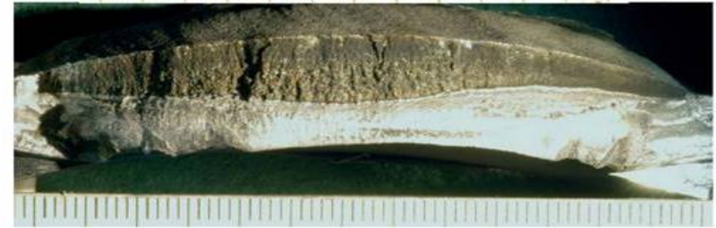
Figure 4. Detected crack on anode pad 16B after the 3 point bending operation (upper image). The crack was forced open and revealed an oxidized fracture surface. The length and depth of the crack was measured to be respectively 76 mm and 8.1 mm.
