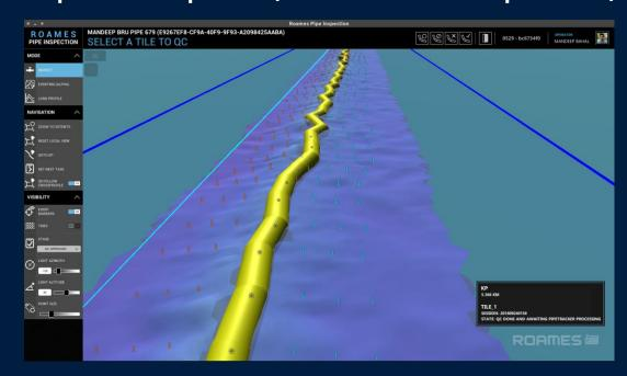
Coarse INS position (grossly exaggerated) uploaded minutes after acquisition
