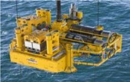
All-electric tree with spring-return actuators.
