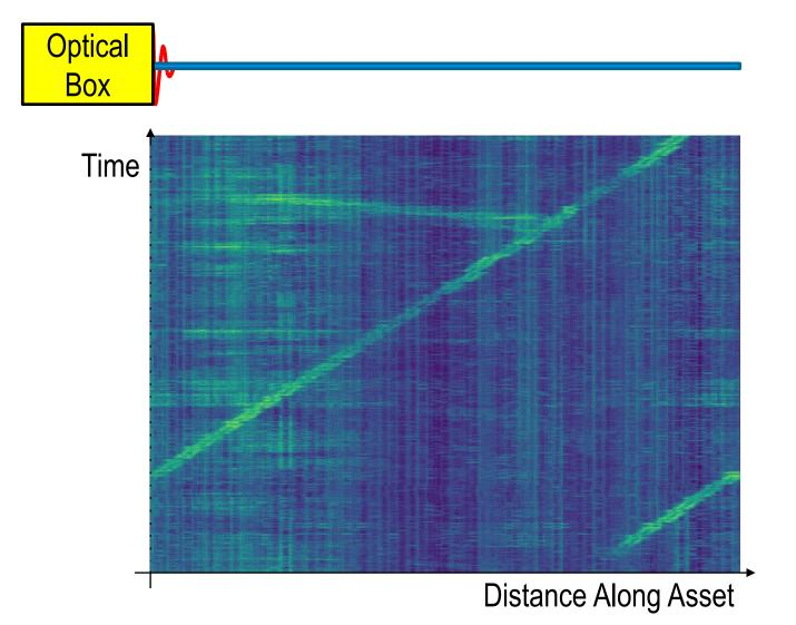
Fibre optic box sends a short pulse into the fibre optic cable
