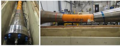
Failed sample after the IP test, where the failure is caused by fiber failure in tension leading to burst of the pipe sample.
