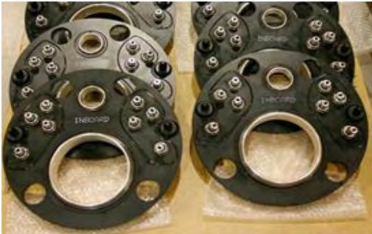
Multibore Seal Plates f/Production, Hydraulics and MEG
