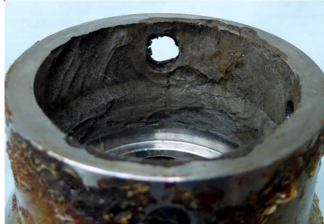
Figure 41 – Corrosion on internal surface and screw threads of back shell
