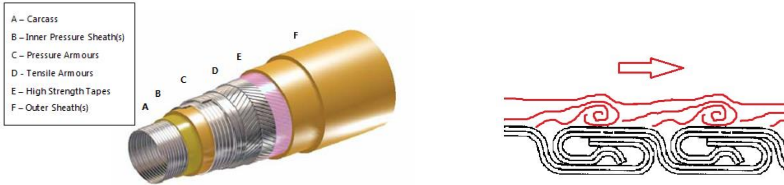
Figure 3-1 Rough Bore Flexible Pipe Cross-section
