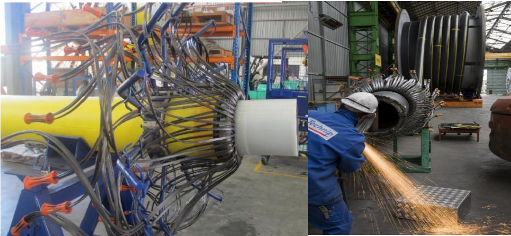
End Fitting mounting process – preparation of flexible pipe layers
