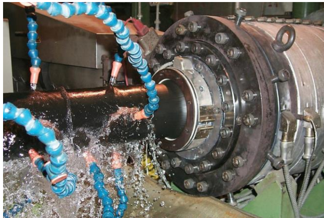
External Sheath Extrusion Process
