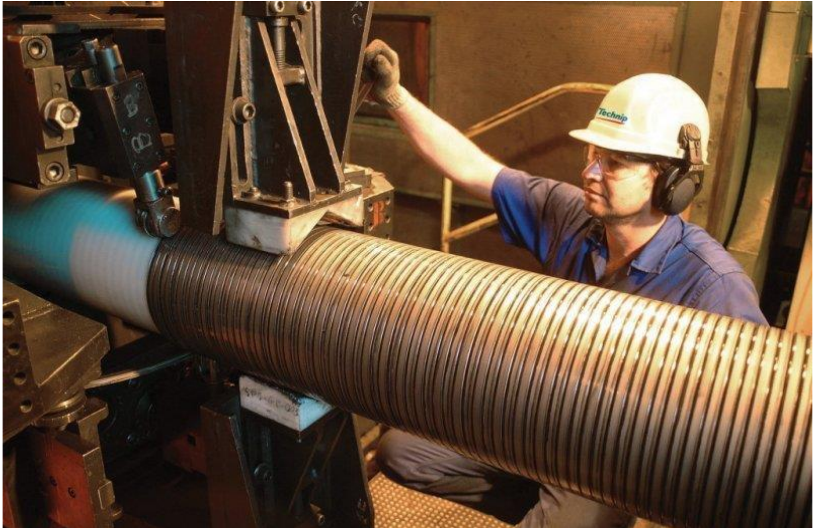
Figure 23 – Pressure Vault Spiralling Process
