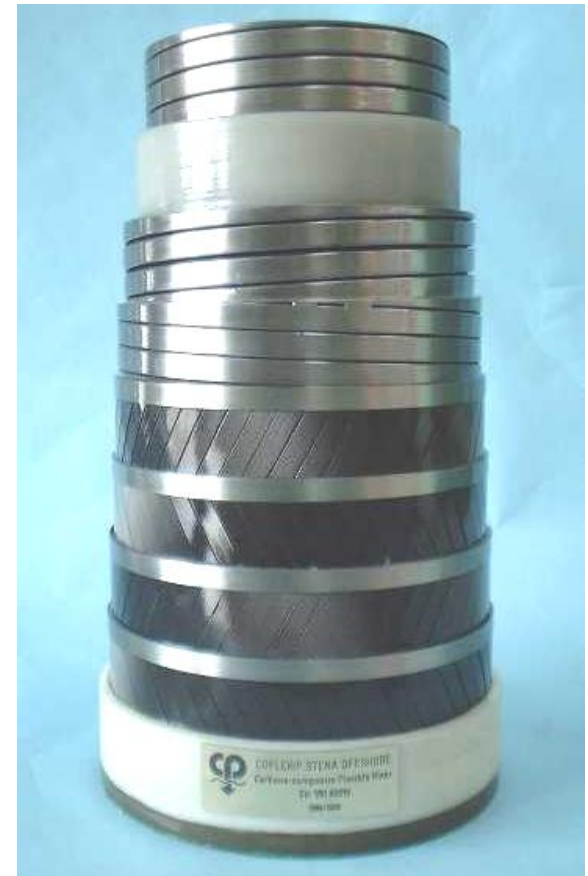
Figure 111 – Carbon Fibre Tensile Armours Structure
