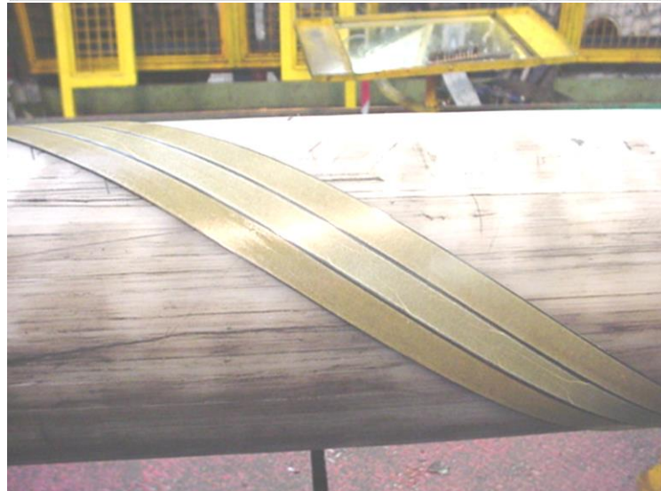
Figure 112 – Carbon Fibre Tensile Armours Structure
