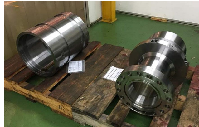
End fitting cover and vault after machining
