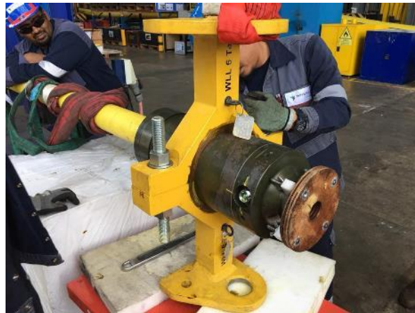
2 part collar for subsea handling
