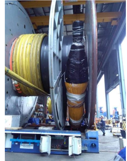
Reel packing with partition
