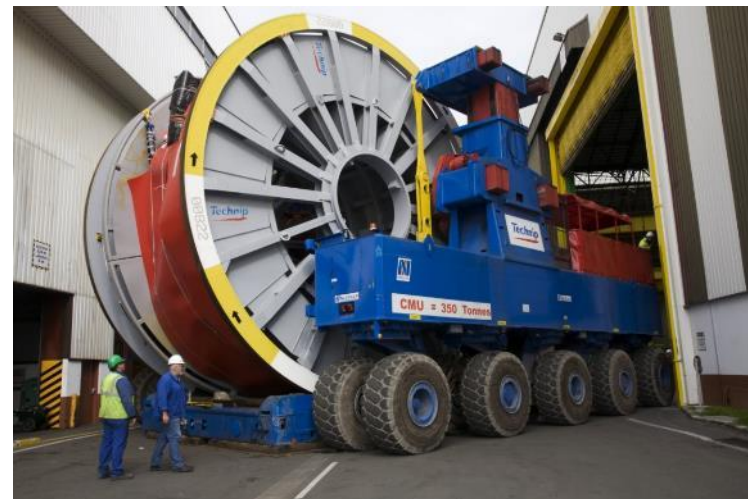
Reel lift and move by Reel Carrier
