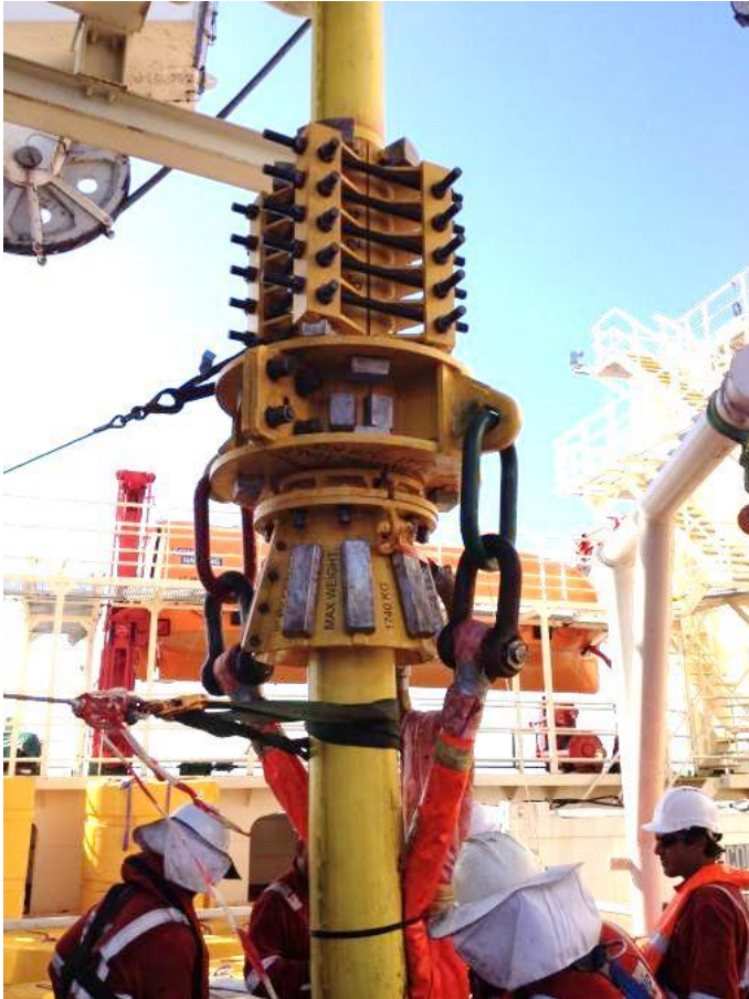
4 part clamp tether Clamp with swivel and dual tether arrangement
