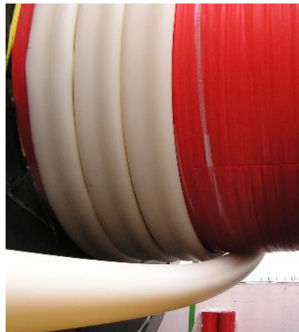
Figure 109 – SB pipe on reel and carousel
