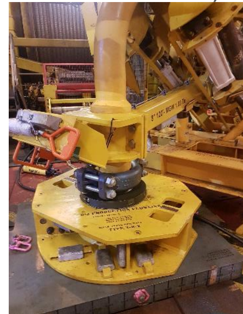
2 part hang-off (installation) collars (before and after installation)
