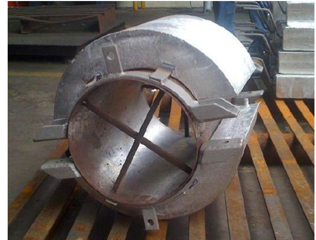
Anode trial fit on mandrel
