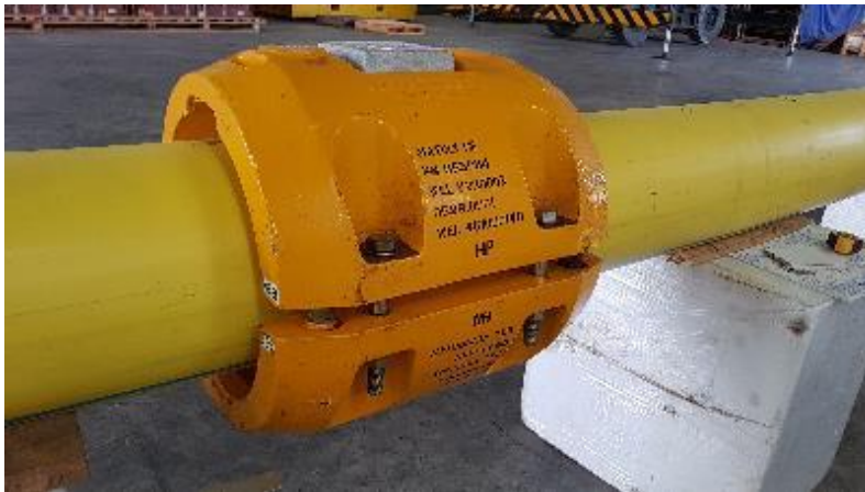
2 part Steel ballast with anodes
