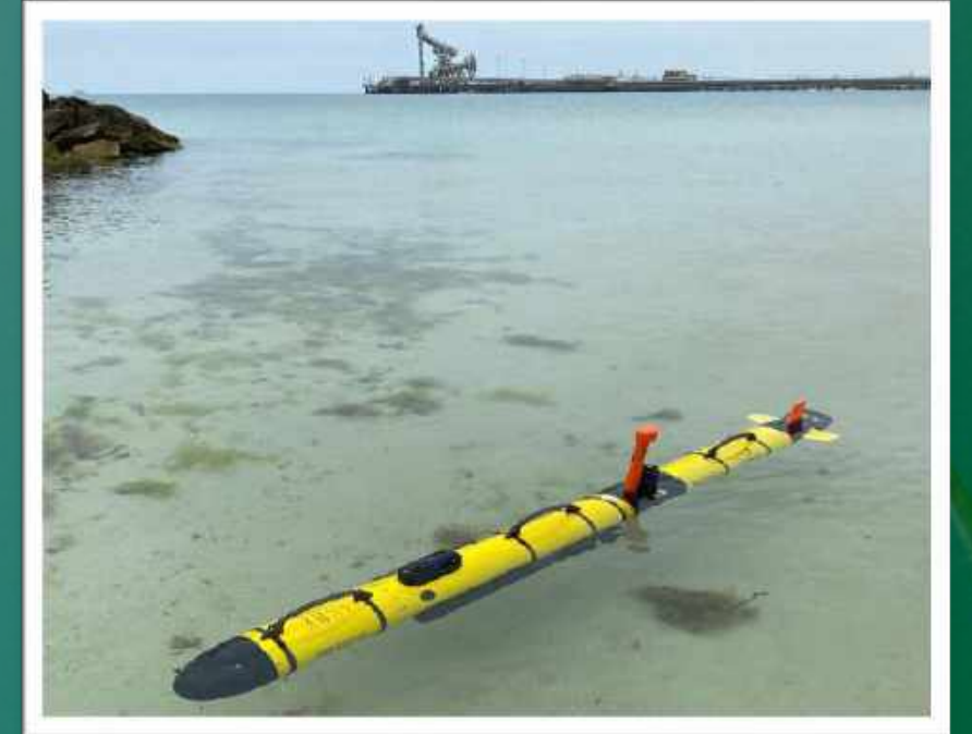
AUV WITH BENTHIC HABITAT SURVEY PAYLOAD
