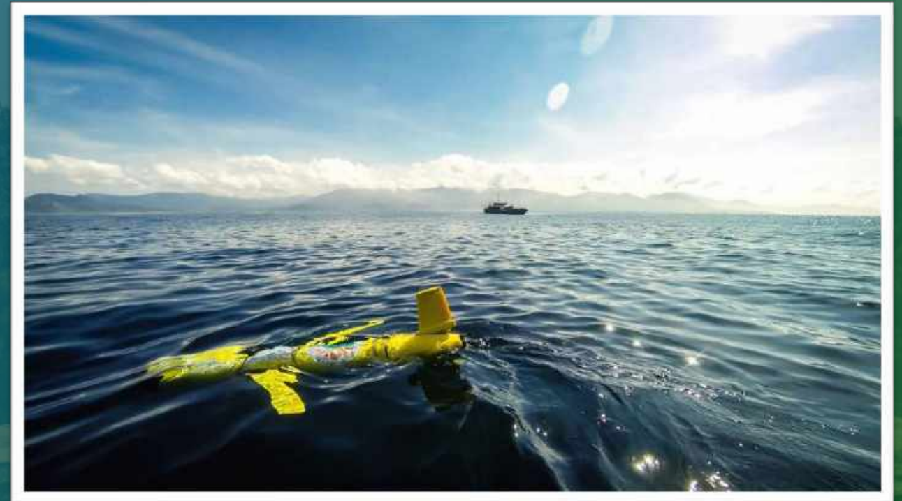
GLIDER DEPLOYED WITH TURBIDITY SENSORS FOR SPOIL DISPOSAL SURVEY
