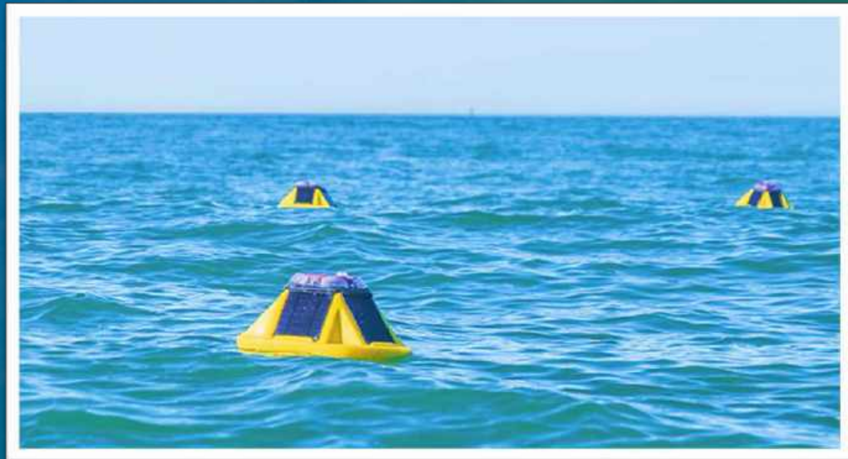
DRIFTING METOCEAN BUOYS WITH REAL-TIME TELEMETRY
