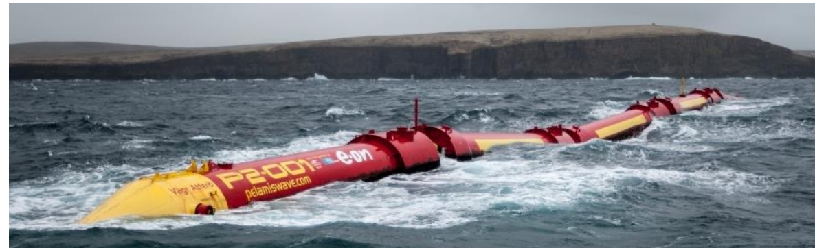
Pelamis's P2 wave energy converter being tested at EMEC – 2010-2014.
