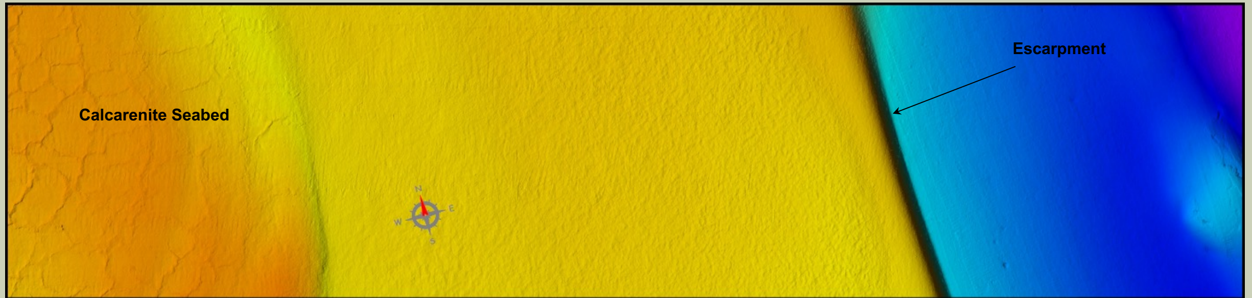
FIGURE 26: MBES DATA SHOWING SEABED TROUGH / NEGATIVE RELIEF & ESCARPMENT
