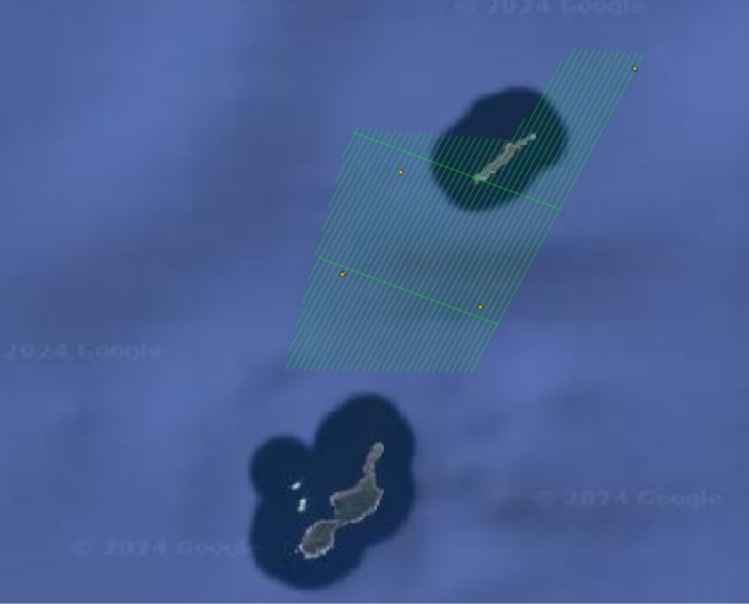
Area and flight lines for aerial magnetometer survey (Thomson Airborne, Google Earth).
